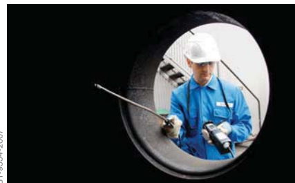
Dräger X-am® 2500 Flexible with external pump for clearance measurements.
