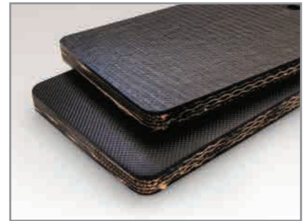
RUB 440 4 PLY, 1/16 x 1/16 SOR-SC-FR (EP600/3 1.5 + 1.5 NBR)
