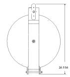
AT 18 7/8" hot products manway for ≤ 14.7 psi working pressure Cover Material Weld Ring Gasket Vent Contact / External
